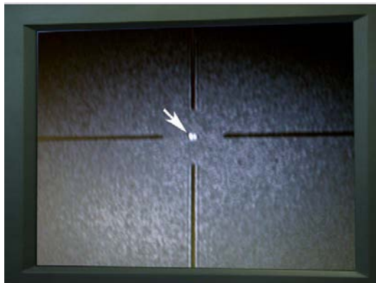
Figure 2. Both the test and reference beams should pass through the crosshairs on the Alignment Monitor.
