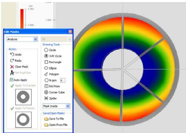
**Figure 3.** Masks can be used to select which data are included in a measurement. This Analysis Mask excludes the support structure for a secondary mirror in a telescope system.
