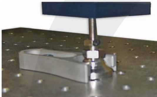
**Figure 1.** Always mount system using swivel feet and kinematic clamps.
