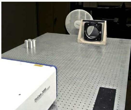
**Figure 4.** Averaging data removes the effect of air turbulence from measurements. Stirring the air with a fan can improve results when the air flow is slow—counter to what you might expect with a standard interferometer.
