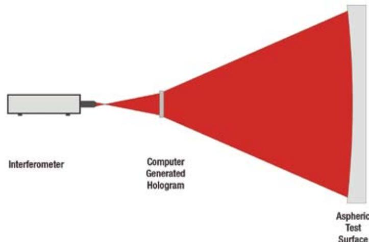
Figure 1. Setup for measuring a large, aspheric optic.
