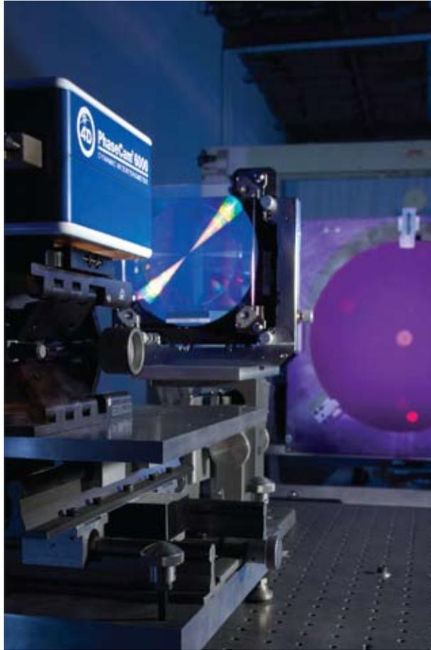
FIGURE 2: Measurement setup for 1.4-meter parabolic optic, with the interferometer in the foreground, CGH and optic. Courtesy Optical Surface Technologies.
