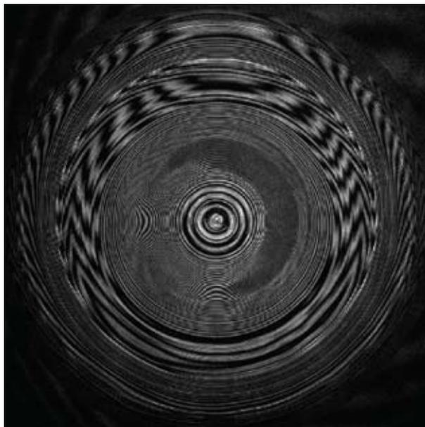
FIGURE 3: Dynamic interferometric measurement of a large aspheric surface during the early stages of polishing.
