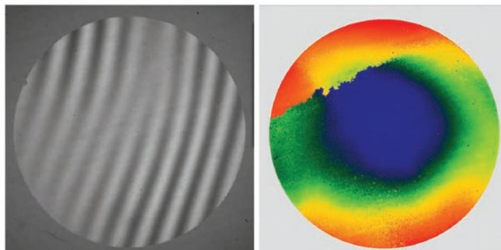
Figure 2. A long Exposure time washes out the fringes (left), leading to unwrapping errors (right). Raise the Gain and lower the Exposure to eliminate this condition.
