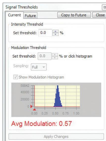
Figure 4. Use the Modulation Histogram to see the effect of the Gain and Exposure settings.
