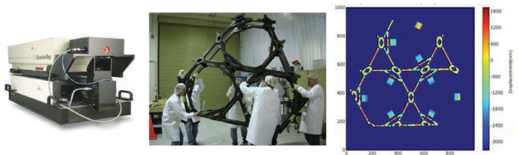
Figure 9. (left) Dynamic ESPI interferometer, (center) JWST backplane sample, (right) ESPI measurement of JWST backplane sample
