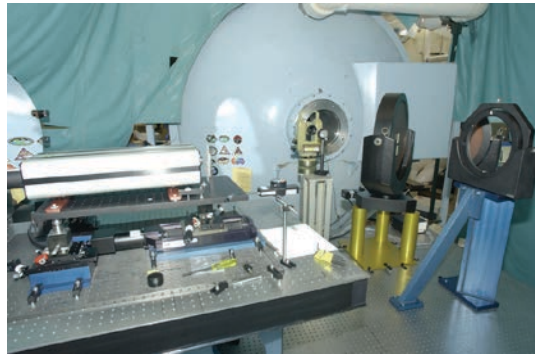
Figure 6. A dynamic interferometer measures a test sample in a vacuum chamber through a view port (Courtesy Ball Aerospace).
