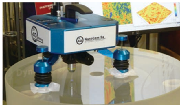
Figure 13. A dynamic interference microscope is immune to vibration, and can be placed anywhere on a large optic without requiring vibration isolation.
