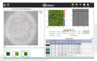
The 4D InSpec quantifies damage, wear and corrosion directly on parts with complex geometries, such as this turbine blade section. Automatic feature finding, 2D traces and 3D plots make it easy to analyze surface features and defects.
